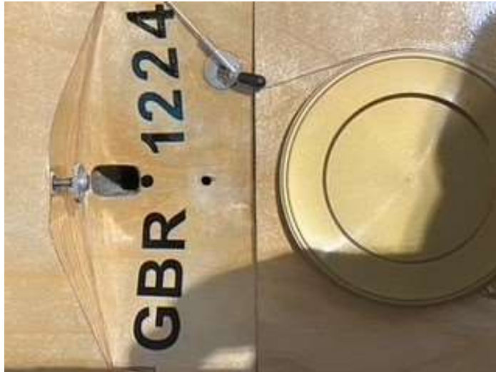
Hull registration number displayed on the external surface of the hull.
